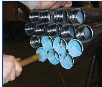
N&N applies anti-gauling thread compound to every rod's pin and box. This also helps reduce torque requirements and wear.
